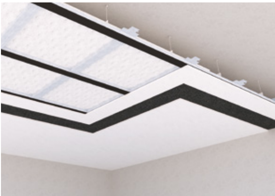
↑ False ceiling with cavity, insertion of insulation material and finishing with double plasterboard
