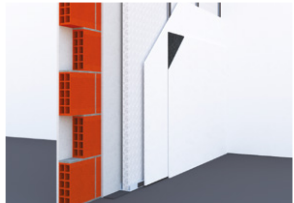
↑ Supporting walls are installed in renovation to increase the soundproofing power of existing walls.
