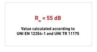
Plaster board wall made of a 50 mm frame with Isolmant Polifibre Bloccarumore and each side sealed by two panels of 12.5mm thick.
