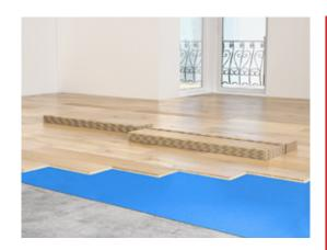
**Preparing the screed.** The surface where ISOLMANT IsolDrum ST BLU is installed should be load-bearing, flat, adequately even, clean and free from debris and oil. However, installer is to assess the suitability of the surface for laying the sheets and the subsequent floating installation of laminate and wooden flooring by carrying out some preliminary checks:
