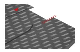
**Installing Isolmant Nastro Alluminio.** Isolmant under screed and under flooring sheets must form a uniform and continuous layer in order to ensure the correct functioning of the floating screed system. It is therefore necessary (especially if they do not have adhesive overlaps and if the continuity of the vapour barrier and thermal insulation is required) to seal them using Isolmant Nastro Alluminio.
