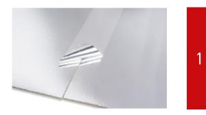
**Installing Isolmant IsolDrum Nastro Alluminato.** Isolmant IsolDrum underlay sheets must form a uniform and continuous layer to ensure the correct functioning of the system. t is therefore necessary (especially if the sheets do not have an adhesive overlapping fabric and if the continuity of the vapour barrier is required) to seal them using Isolmant IsolDrum Nastro Allunminato, cutting it to size as needed with a normal construction site cutter.
