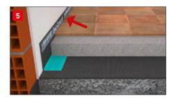
**Installing Fascia Tagliamuro.** Before installing all the partitions, Isolmant Fascia Tagliamuro must be laid. This high density,reticulated polyethylene foam accessory is specifically designed to disjoint partitions and slabs, thereby helping to reduce the structural sound transmission from the walls to the slab. This product is available in different thicknesses and densities depending on the weight of the partitions (Fig.1)
