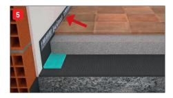
**Installing Fascia Tagliamuro.** Before installing all the partitions, Isolmant Fascia Tagliamuro must be laid. This high density reticulated polyethylene foam accessory is specifically designed to disjoint partitions and slabs, thereby helping to reduce the structural sound transmission from the walls to the slab. This band is available in different thicknesses and densities depending on the weight of the partitions (fig. 1).
