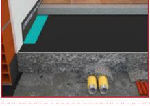
**Installing Fascia Tagliamuro.** Before installing all the partitions, Isolmant Fascia Tagliamuro must be laid. This high density, reticulated polyethylene foam accessory is specifically designed to disjoint partitions and slabs, thereby helping to reduce the structural sound transmission from the walls to the slab. This product is available in different thicknesses and densities depending on the weight of the partitions (Fig.1)
