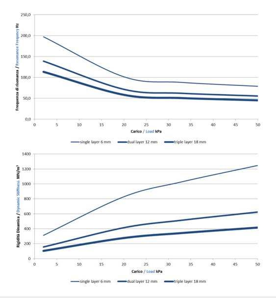
Variation in resonance frequency and dynamic stiffness as a function of load, for different layers of Isolmant Strong.
