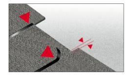
**Installing Isolmant Nastro Telato.** Isolmant underlay range sheet must form a uniform and continuous layer in order to ensure the correct functioning of the floating screed system. If the sheets do not have adhesive overlaps to seal them with Isolmant Nastro Telato.
