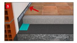
**Installing Fascia Tagliamuro.** Before installing all the partitions, Isolmant Fascia Tagliamuro must be laid. This high density,reticulated polyethylene foam accessory is specifically designed to disjoint partitions and slabs, thereby helping to reduce the structural sound transmission from the walls to the slab. This product s available in different thicknesses and densities depending on the weight of the partitions (fig.1)
